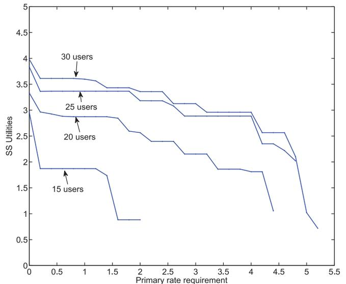
Fig. 8. Comparison of the SS utility objectives for different number of nodes ( $K = 10, 15, 20, 25$ , and  $30$ ) with the increasing rate requirements for the primary sessions.
