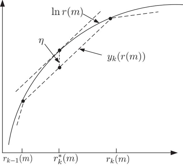
Fig. 3. An illustration of the maximum approximation error for piece-wise linear segment.
